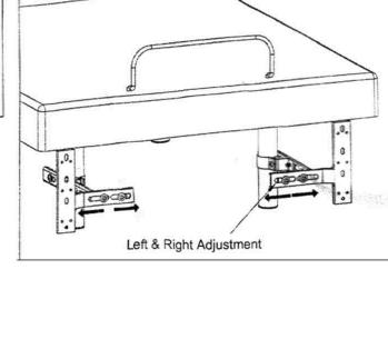
2 Use the Allen Key (D) to loosen the circle elip bolts, attach the circle clip to the leg, when you adjust to the right position to fit the headboard bolts hole, tighten up the bolts again. If can't match headboard bolts hole, please move to next step.
