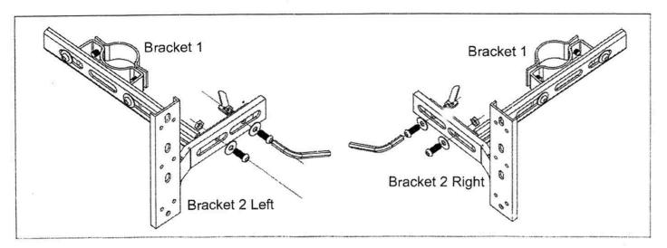
1 Please use 2 Bolts (A), 2 Spacers (B), and 2 Nuts (C) to connect Bracket 1 (F) and Bracket 2 (G) by Allen Key (D), but do not tighten.
