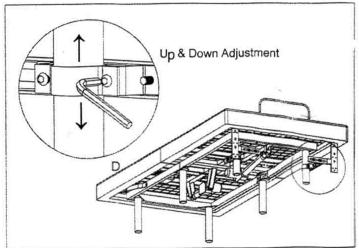
3 Loosen the bolts as shown. Move the Bracket to match the headboard bolts hole, then tighten up the bolts.
